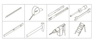
drills hammer drill, ladder/scaffolding, screwdriver, hammer measure tape, pencil/marker, spirit level, ring/flat wrenches, Allen keys, anchors.
