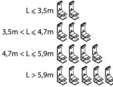
It is recommended to mount the outer wall brackets at a distance of 20 to 45 cm from the ends of the awning, and place the remaining brackets at equal intervals.
